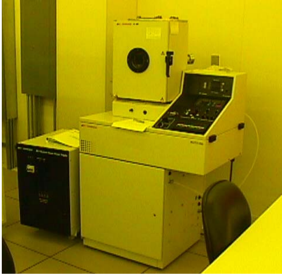
Figure 42 Electron beam evaporator located in the AFIT cleanroom.
