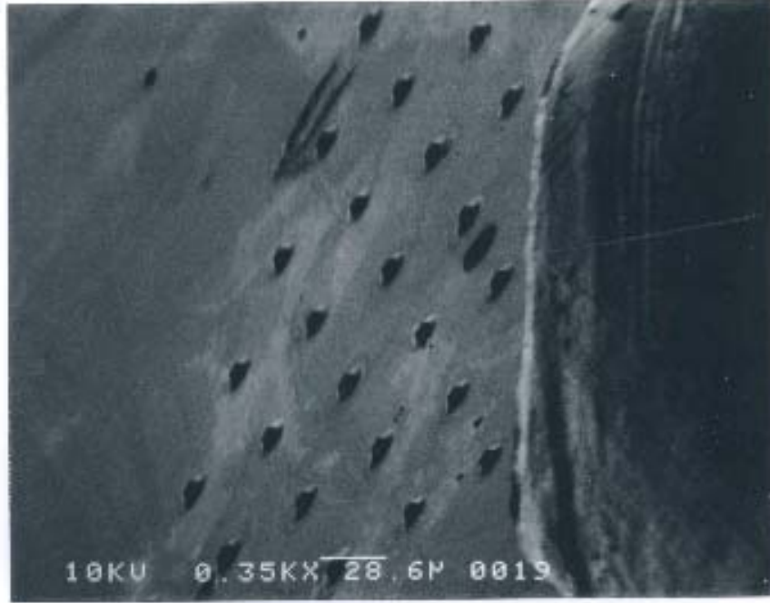
Figure 55 SEM photo (350x) of mesas after wet etch.
