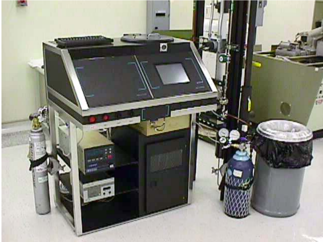
Figure 44 Phantom RIE system [5].
